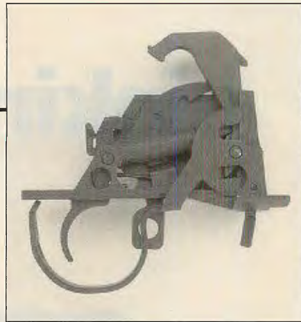
M14/M1A trigger assembly, (left) shown here with the hammer cocked and the trigger guard down for disassembly purposes, was lifted right out of the .30 M1 Garand. (right) M14/M1A trigger assembly with the hammer forward in the fired position.
